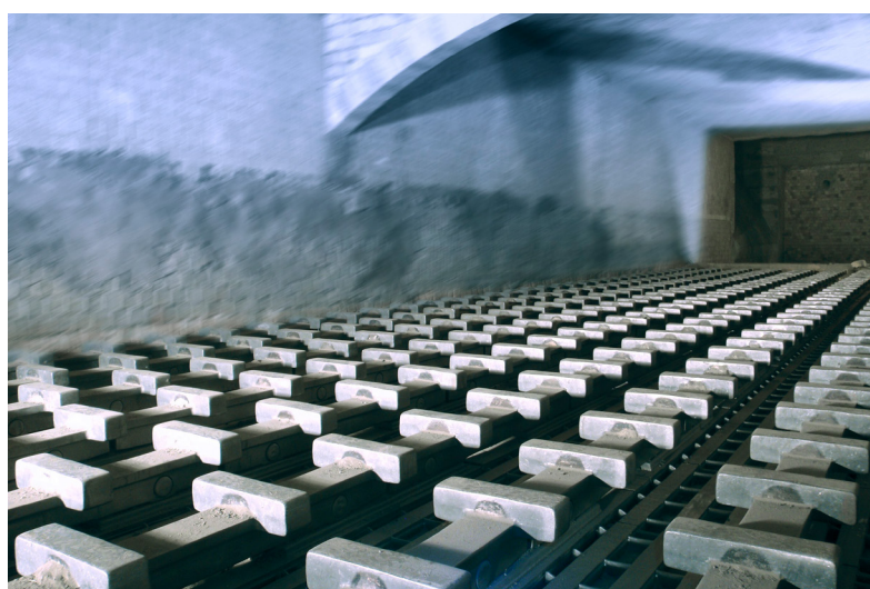
Figure 2: thyssenkrupp’s POLYTRACK conveyor system cools and transports the cement clinker.
