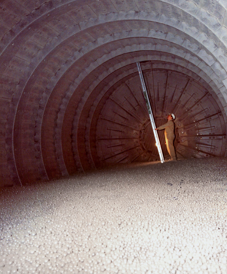
Figure 3: The grinding of the cement by means of balls in a pipe mills.
