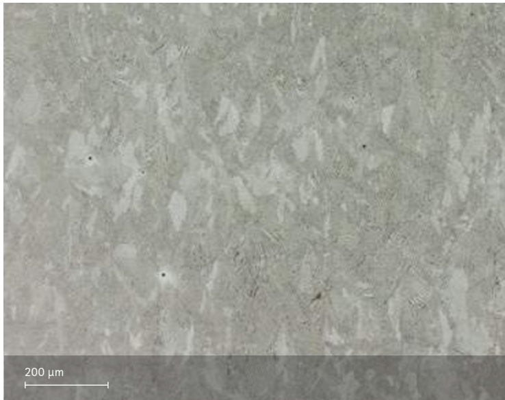
Heat treated microstructure. Etched with Kalling's II etchant.
