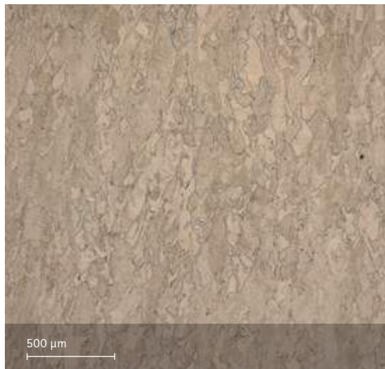
Microstructure solution annealed Etched with etchant Kallings 2
