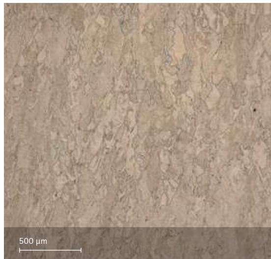
Microstructure solution annealed Etched with etchant Kallings 2
