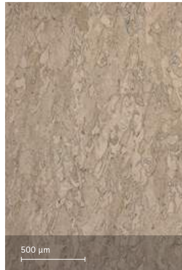
Microstructure solution annealed Etched with etchant Kallings 2
