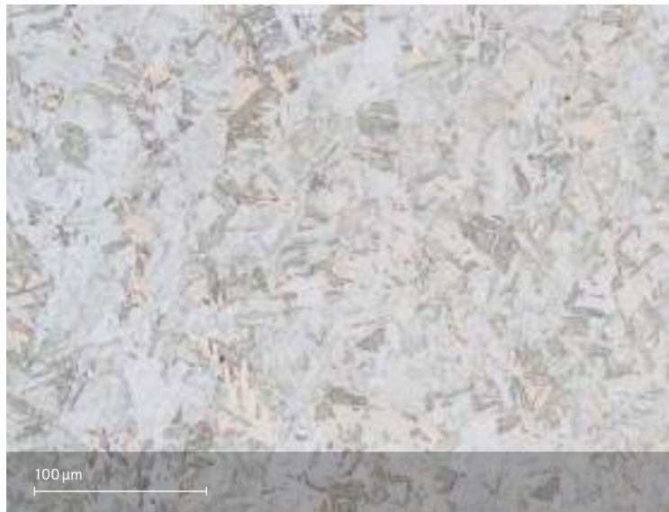
Heat treated microstructure. Etching; ASTM E407-94
