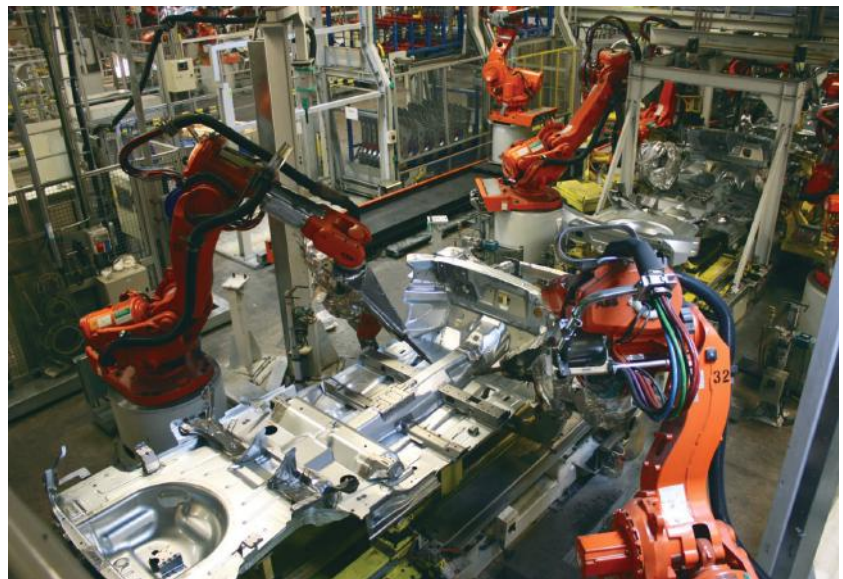
Volvo Cars Torslanda plant floor subassembly line – V70 floor follows a V60 floor – a physical line.
